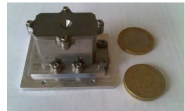
Highly Miniaturised Radiation Monitor (HMRM) [RAL, UK]
